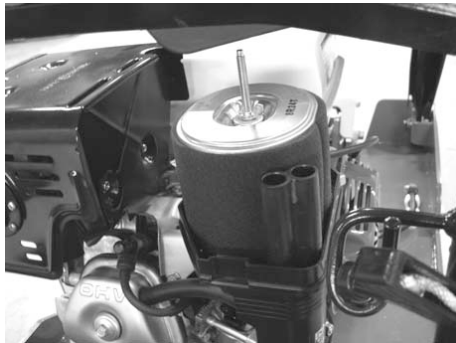
Fig. Replacing air filter.
