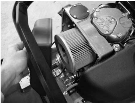
Fig. Replacing air filter.
