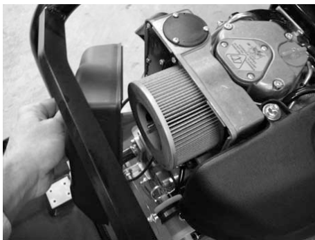
Fig. Replacing air filter.
