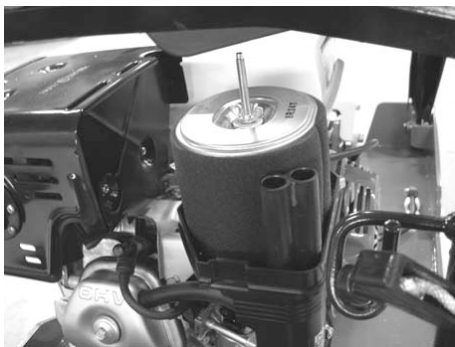
Fig. Replacing air filter.
