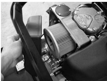
Fig. Replacing air filter.
