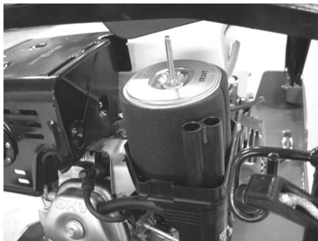
Fig. Replacing air filter.
