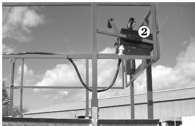
Figure 6.1.2 - Control Box Location, Platform Position
