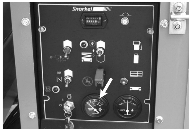
Figure 4.1 - Water Temperature Gauge
