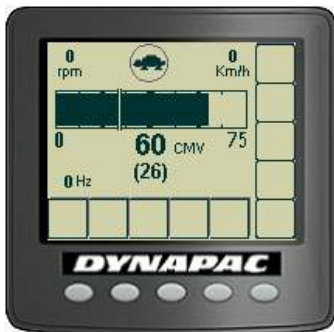
Fig. Compaction meter display (CMV display)
