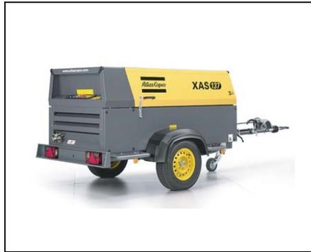
The compressors type XA(S) 137 DD - XA(S) 300 DD7, XA(S) 137 DDG - XA(S) 300 DD7G and XAHS 107 DD - XAHS 250 DD7 are silenced, single-stage, oil-injected screw compressors, built for a nominal effective working pressure, ranging from 7 bar (101.5 psi) up to 12 bar (174 psi) (see chapter **Technical specifications**).
