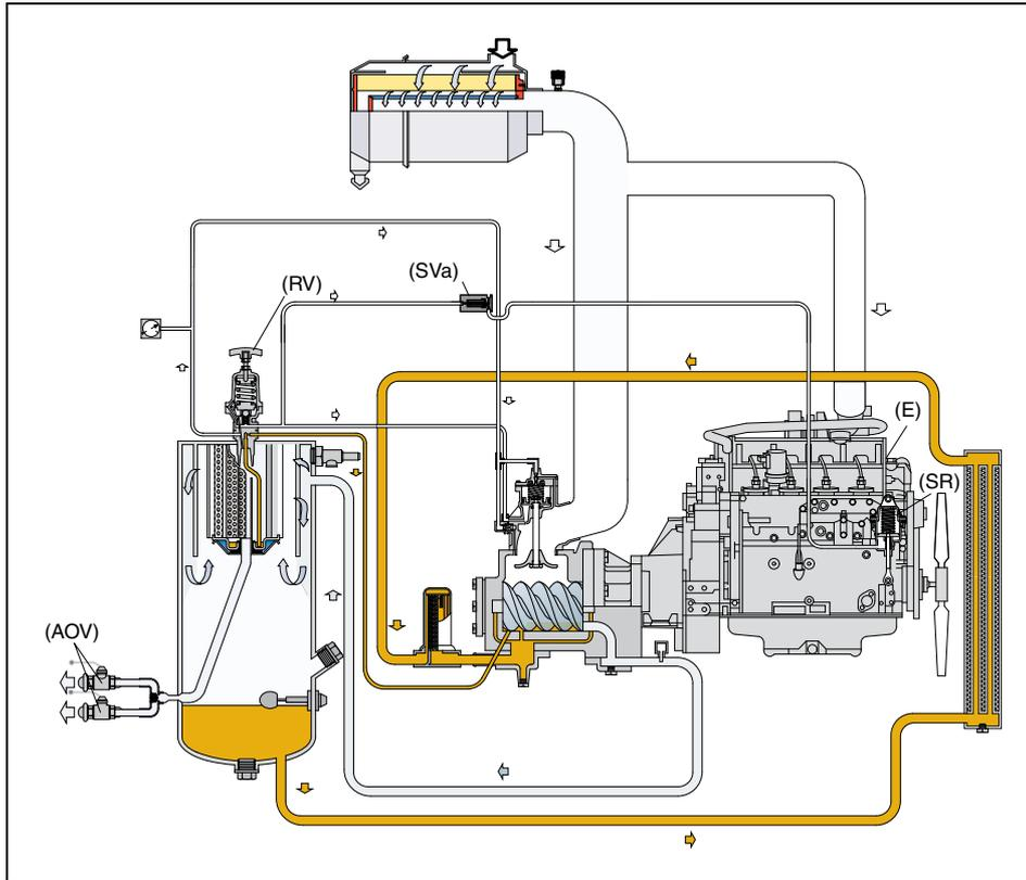
The working pressure is determined by the tension of the spring in the regulating valve (RV). This tension can be increased to raise the pressure and decreased to lower it by turning the adjusting wheel clockwise and anti-clockwise respectively.
