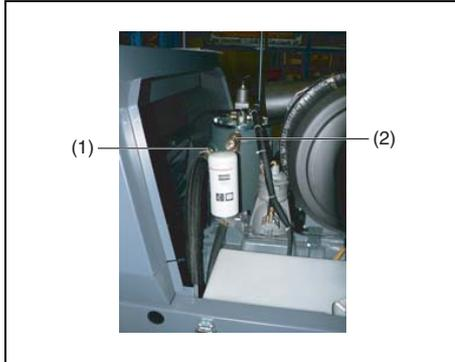
The air receiver (1) is tested according to official standards. Regularly have inspections carried out in conformity with local regulations.
