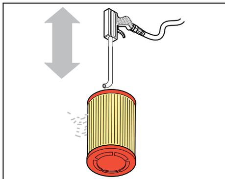
Next carefully examine the element for possible damage. Never beat or knock the element as this will damage it and there will be a danger of damage to the engine.
