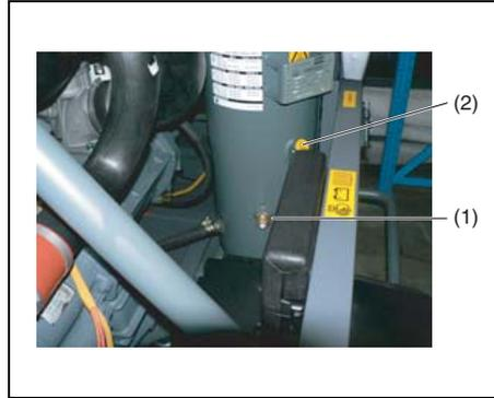
With the unit standing level, check the level of the compressor oil. The pointer of the oil level gauge (1) must register in the upper extremity of the green range. Add oil if necessary.
