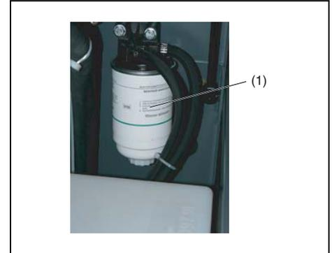
Replacing the filter element
