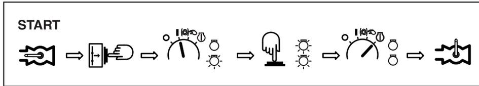
1. To start, turn start switch S1 clockwise to position 1, lamp H2 (general alarm lamp) will go on.
