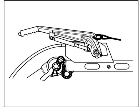
*Hand brake lever downward - brake not operated*
