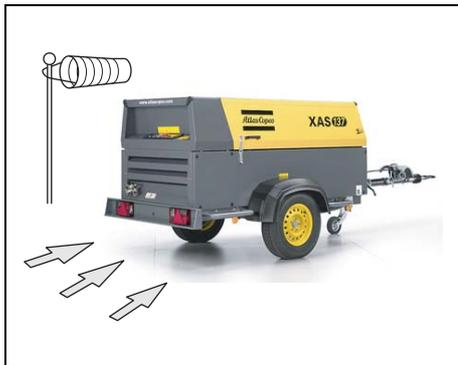
Locate the rear-end of the compressor upwind, away from contaminated wind-streams and walls. Avoid recirculation of exhaust air from the engine. This causes overheating and engine power decrease.
