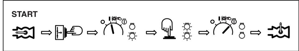
1. To start, turn start switch S1 clockwise to position 1, lamp H2 (general alarm lamp) will go on.
