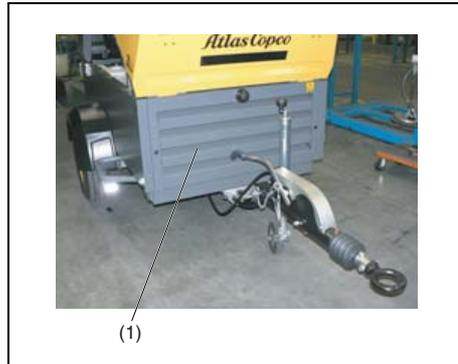
Keep the coolers clean to maintain the cooling efficiency.
