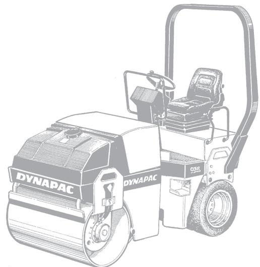
*The CC 102/122 and CC 132 are specially designed for repair work on asphalt compounds, but can also be used for paving small streets, sidewalks and bicycle trails. They are often used as a complement to bigger rollers for compacting cross-joints and restricted spaces.*
