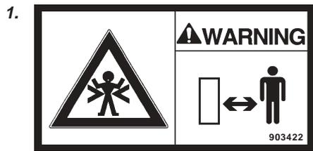
Crush zone, articulation/drum. Maintain a safe distance from the crush zone.
