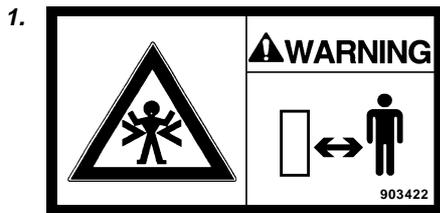
**1.** Crush zone, articulation/ Drum. Maintain a safe distance from the crush zone.
