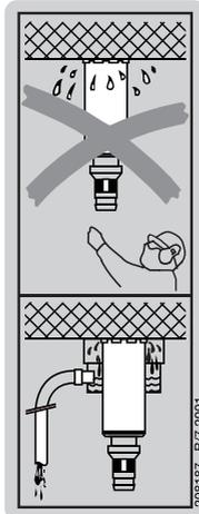
Use of the water collector system in conjunction with a wet-type vacuum cleaner is mandatory when working overhead on ceilings.
