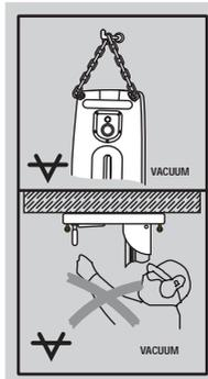
Overhead drilling with the drill stand attached only by vacuum is not permissible.
