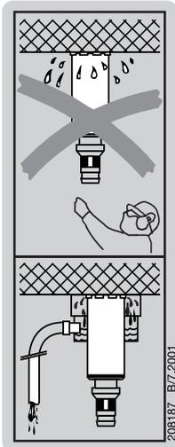
Use of the water collection system in conjunction with a wet-type vacuum cleaner is mandatory for overhead drilling. Position the side handle and water swivel / extraction head so that the water collection system can be fitted without obstruction. The centering ring and seal must be of a size suitable for the core bit diameter used.
