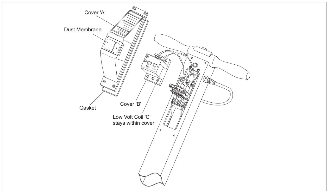
6. Using standard procedure test for electrical safety (Class 1 Earthed Appliance [U.K.] ). Do not exceed 1250 volt flash duration of 3 seconds.
