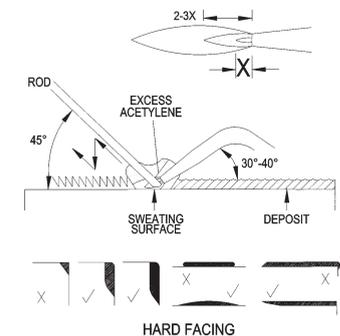
2. Use a carburising oxy-acetylene flame with the acetylene feather 2 or 3 times the length of the inner cone. The inner cone of the flame is held about 3 mm from the surface until the surface 'sweats'.
