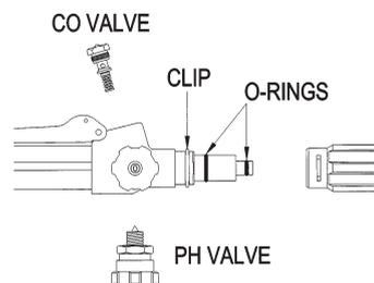
4. If the cutting oxygen valve will not snap closed or is leaking fold back
