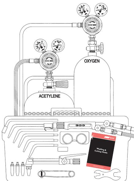
**BOC's ProMaster, Master and MasterStart kits**, in conjunction with cylinders of oxygen and acetylene, provide a comprehensive set of metalwork tools. This plant will provide:
