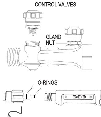
2. Check the condition of both o-rings on the mixer by removing the hook and sliding the nut to expose the o-rings. If they are chipped or worn remove the o-rings with a clean narrow blunt tool that will not damage the metal grooves. Roll in new replacement o-rings and twist to seat in the groove.
