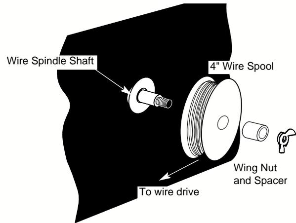
**Note:** The brake should be adjusted with a spool of wire installed. When properly adjusted it should move freely but not coast.
