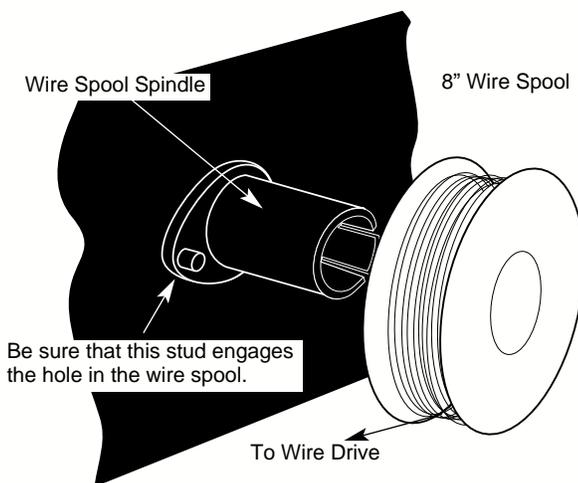
Wire Spool must be pushed all the way on the spindle so that the spindle's tab will hold it in place. The Wire Spool will rotate clockwise when wire is dereeled.
