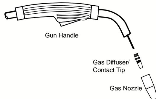
12. Replace contact tip and gas nozzle.
