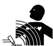
**ELECTRIC AND MAGNETIC FIELDS — May be dangerous. Electric current flowing through any conductor causes localized Electric and Magnetic Fields (EMF). Welding and cutting current creates EMF around welding cables and welding machines. Therefore:**
