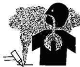
**FUMES AND GASES -- Fumes and gases, can cause discomfort or harm, particularly in confined spaces. Do not breathe fumes and gases. Shielding gases can cause asphyxiation.**
