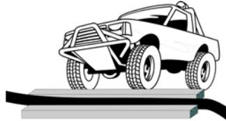
Prevent hydrostatic shock by using thick planking either side of the hose where it crosses roadways.
