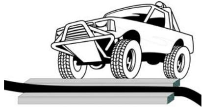
Prevent hydrostatic shock by using thick planking either side of the hose where it crosses roadways.
