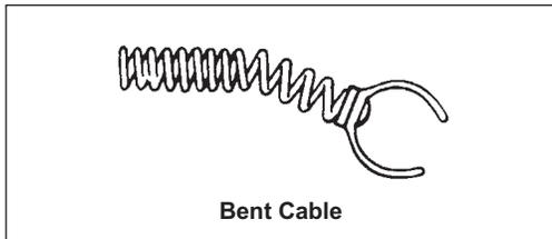
Figure 10 – Bending Cable for Faster Cleaning
