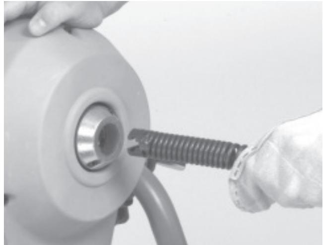
**Figure 4 – Inserting Cable Into Front Of Machine**
